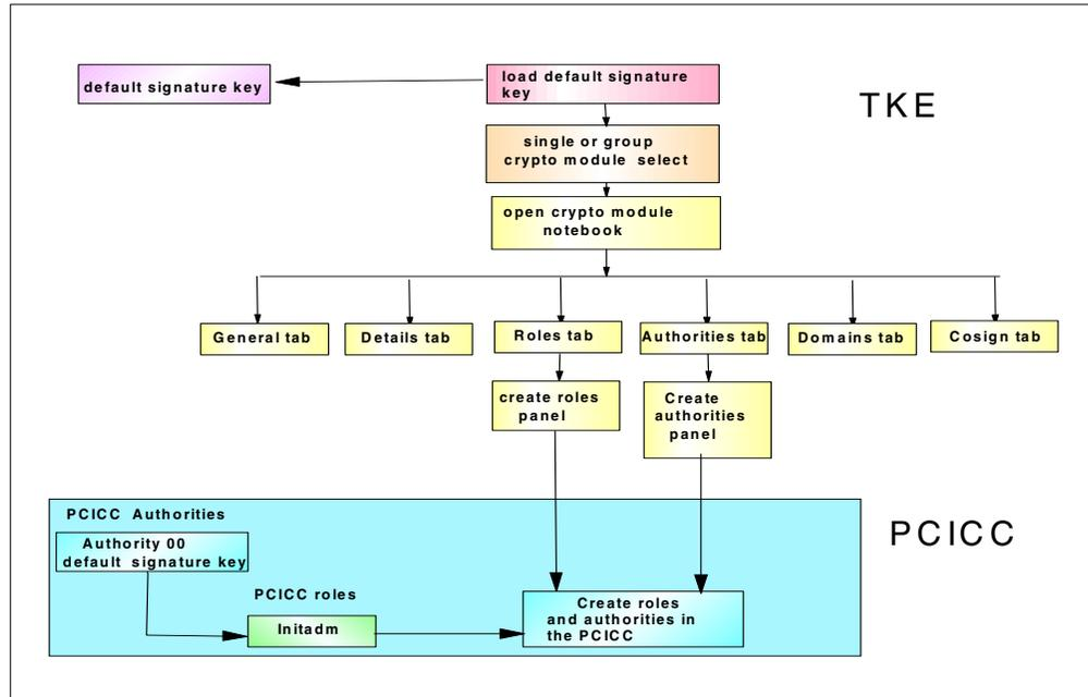
Figure 82. PCICC initial role & profile after new card install or card zeroize from SE
