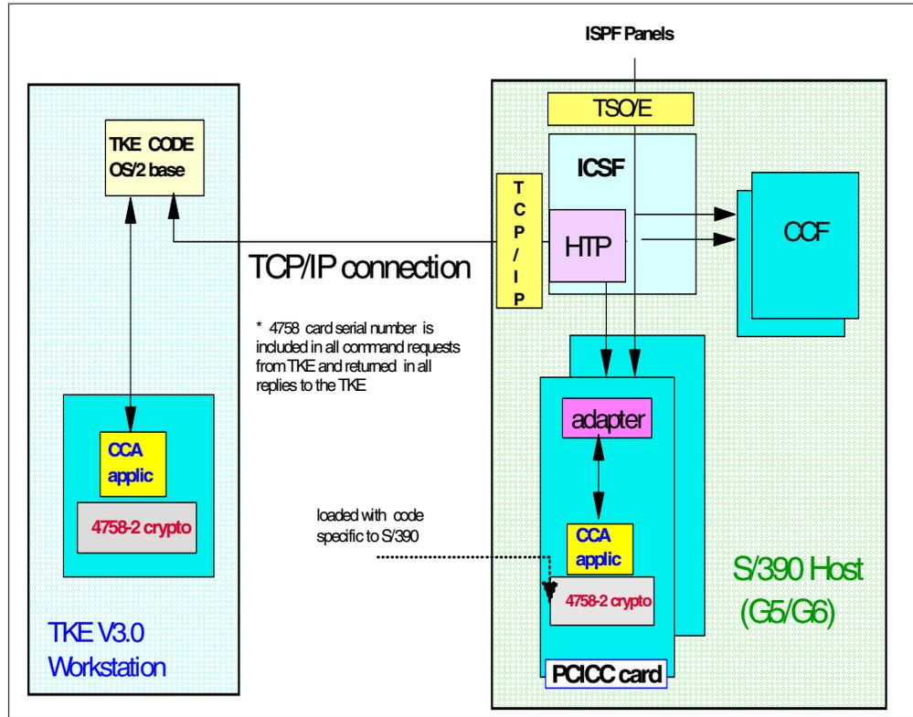
Figure 59. TKE workstation and host system
