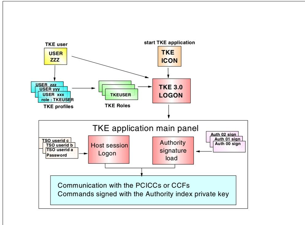
Figure 72. Host Crypto module access logon sequence from TKE
