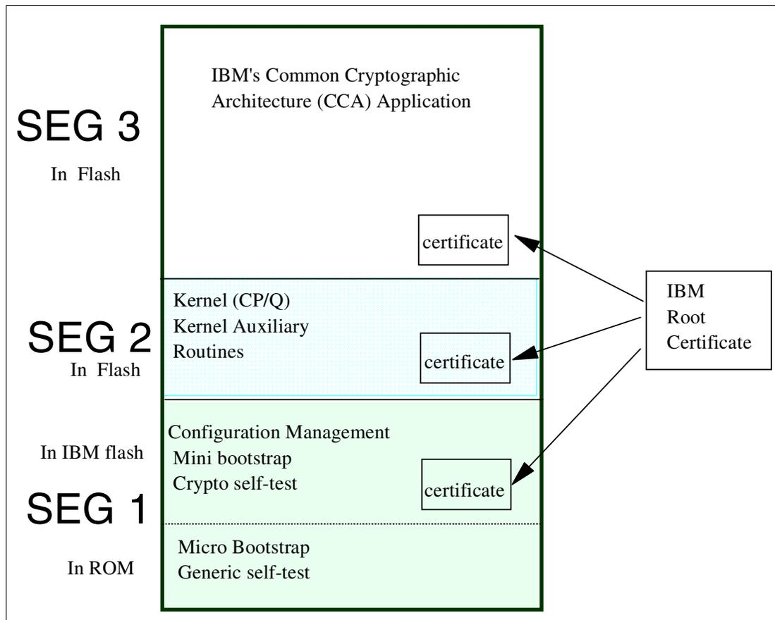
Figure 10. Crypto software architecture in the IBM 4758 Technology
