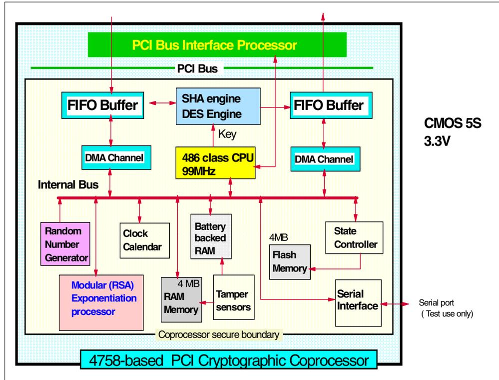
Figure 5. 4758-based Crypto coprocessor hardware data flow
