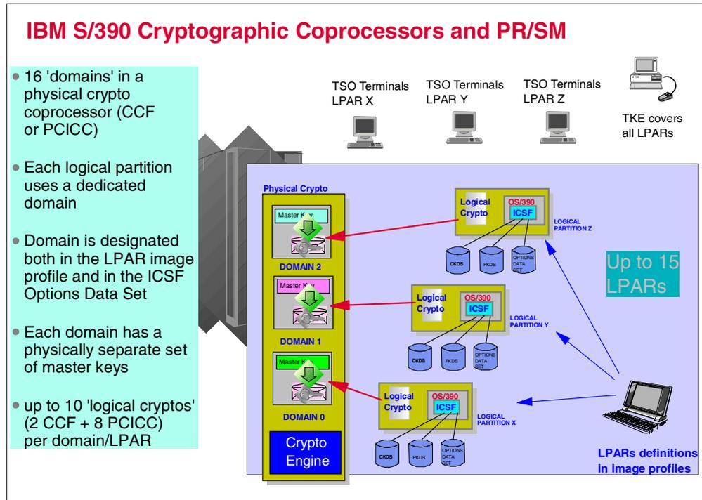
Figure 3. Physical coprocessor domains and logical coprocessors
