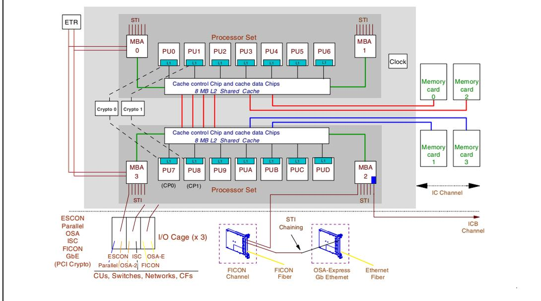
Figure 18. 9672 G6 internal system structure
