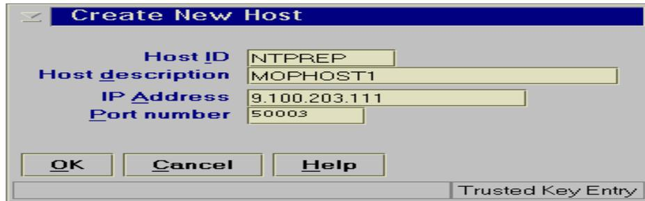
Figure 76. Create a new host panel on TKE workstation example: NTPREP
