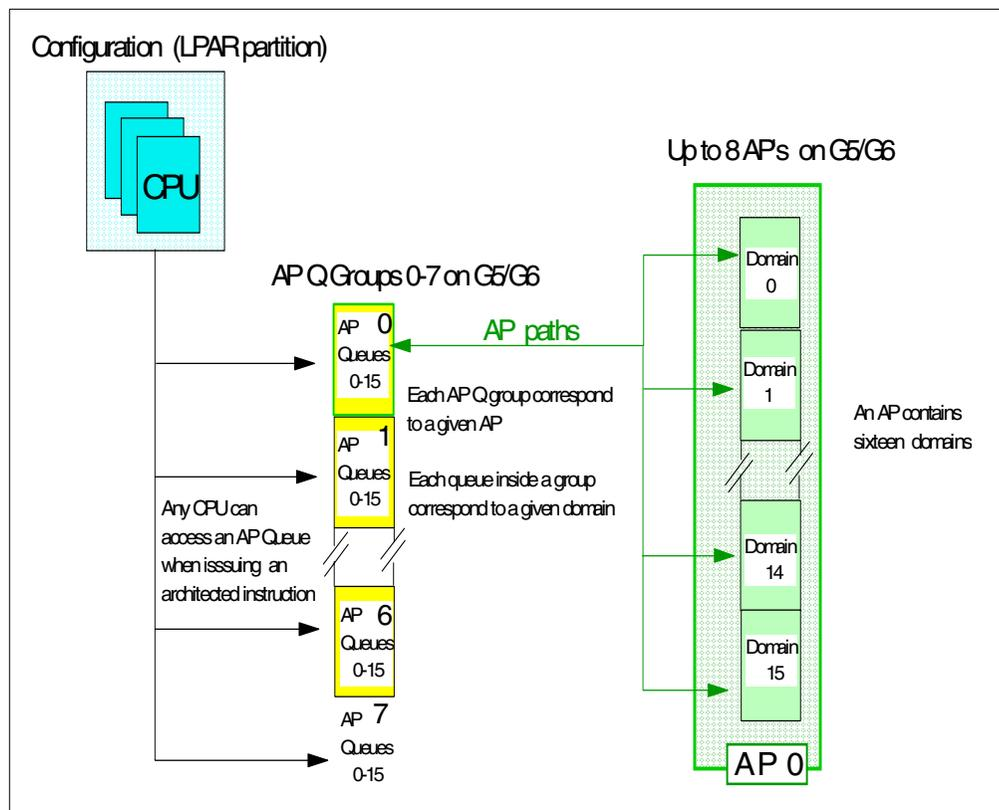
Figure 9. AP architecture: high-level view
