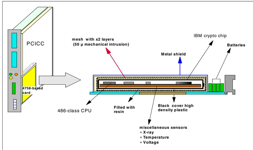
Figure 8. 4758-based card on S/390: longitudinal section
