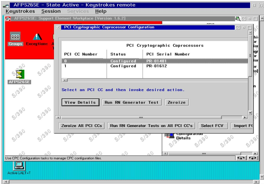
Figure 14. PCI CC status after FCV selected and CHPID configured online
