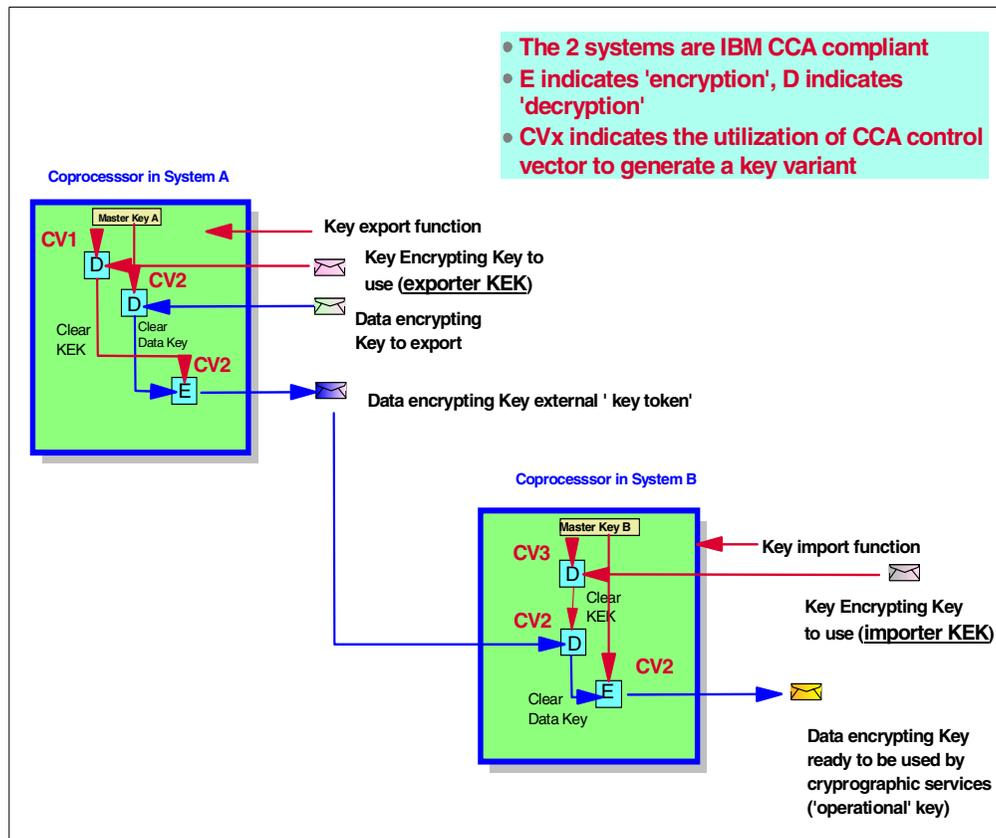
Figure 1. Example of IBM CCA Master Key and key separation concepts
