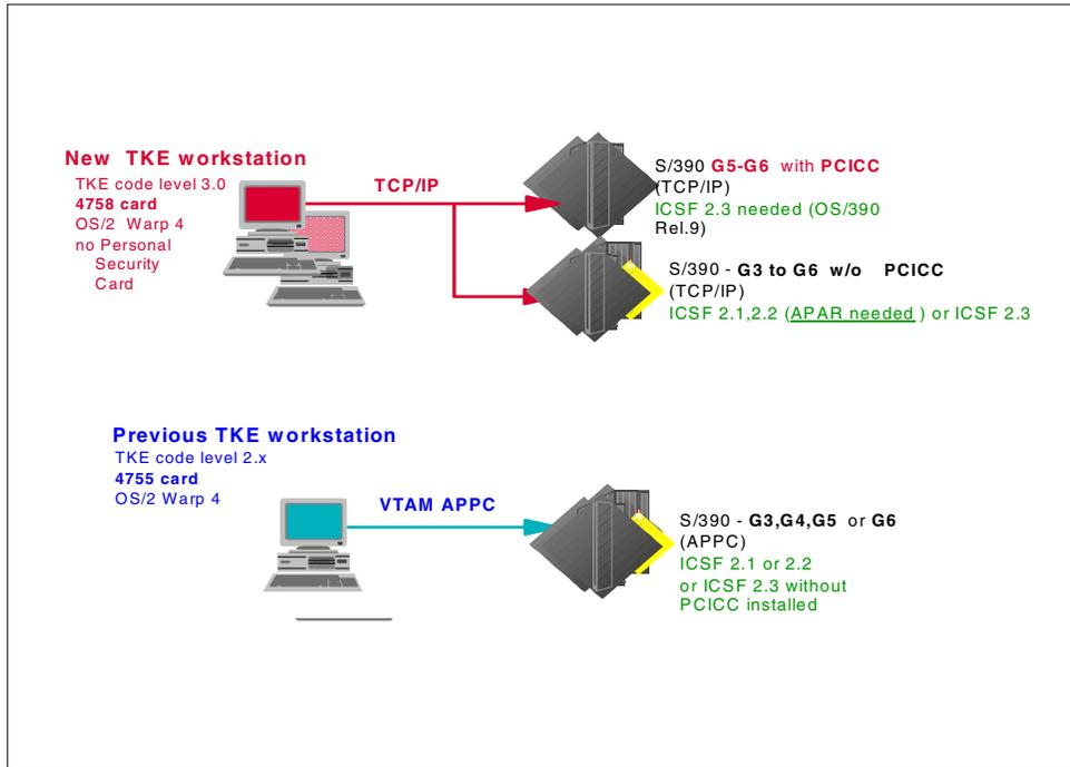
Figure 58. TKE workstation configuration according to CMOS models
