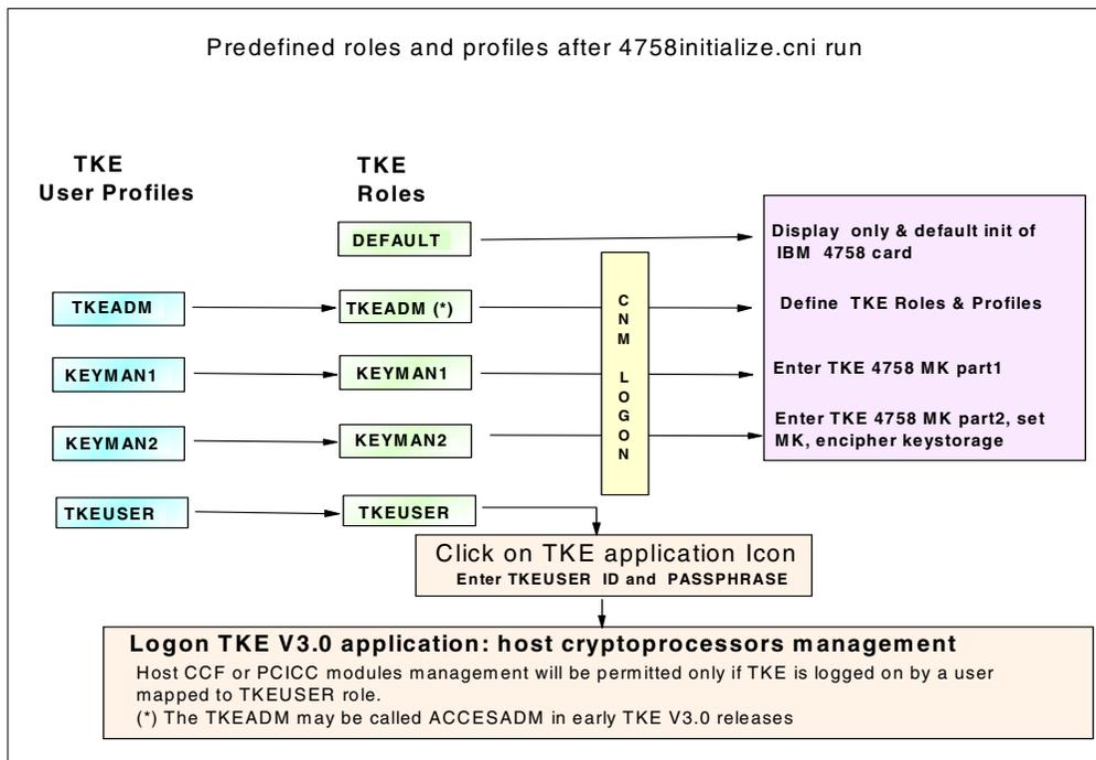
Figure 64. TKE workstation predefined roles and profiles
