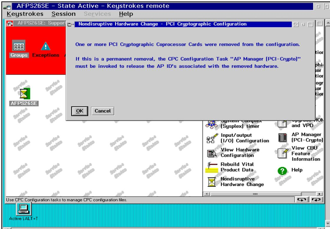
Figure 16. Msg. after PCICC Card removed by Nondisruptive Hardware Change
