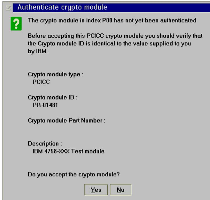
Figure 78. New Crypto module authentication panel
