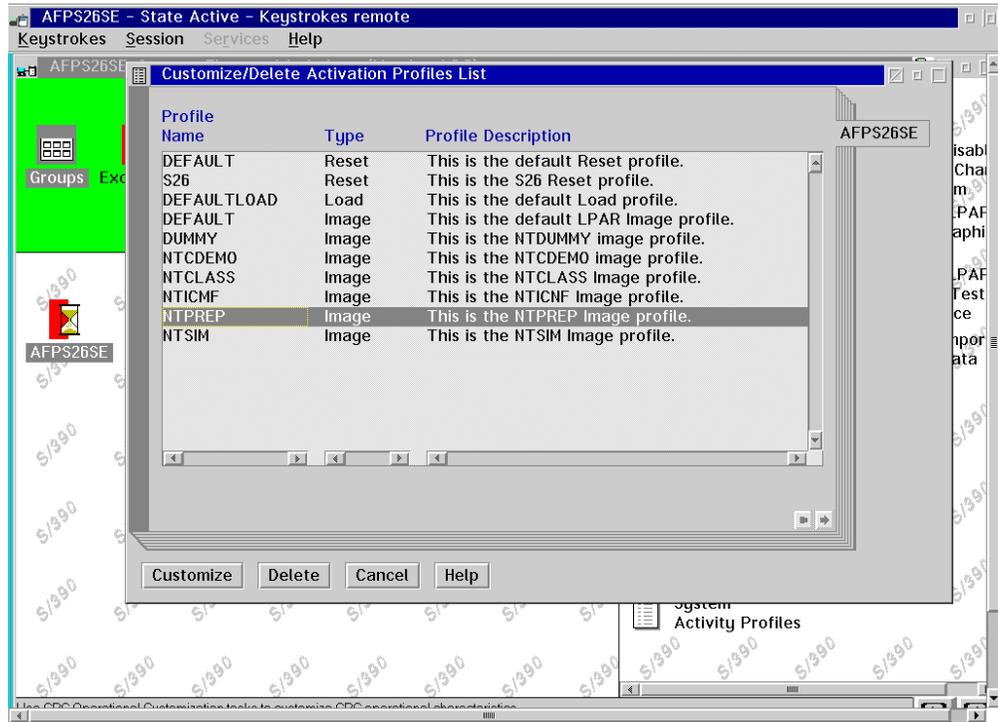
Figure 26. The Activation Profiles List
