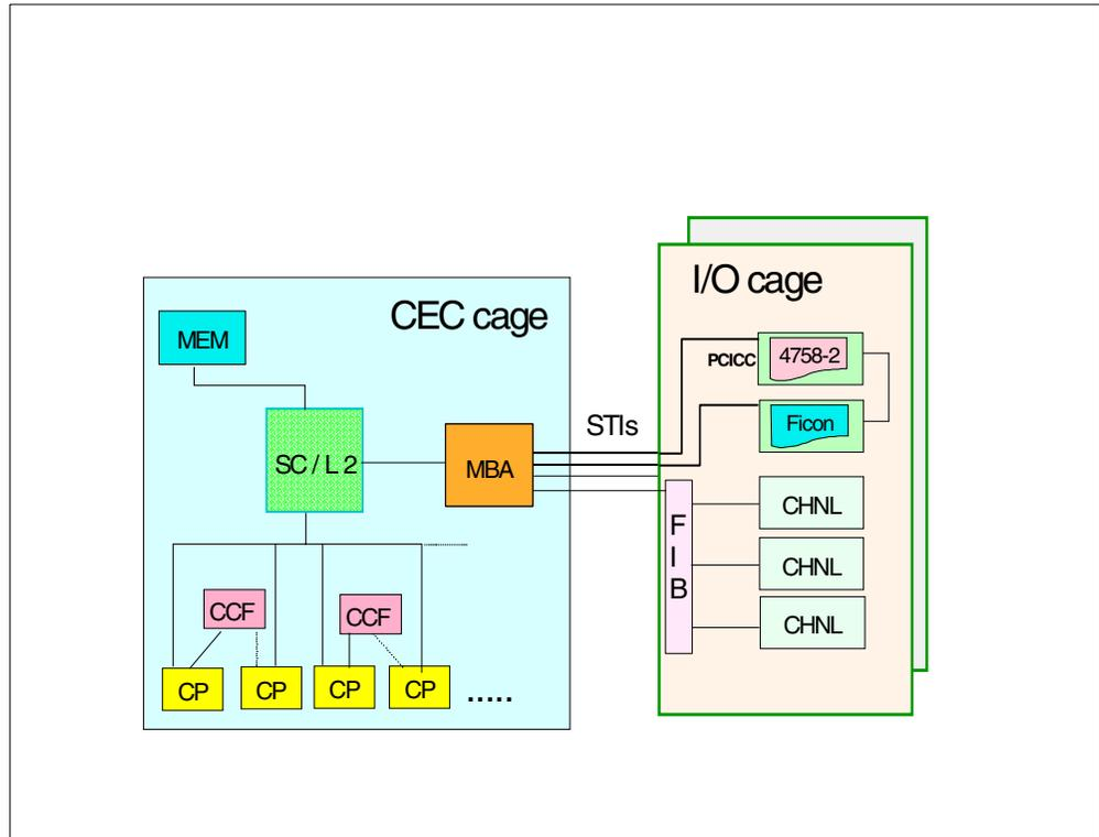
Figure 4. CCF and PCICC hardware data flow on S/390 G5/G6
